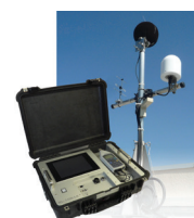
Automatic measuring system for aircraft noise
